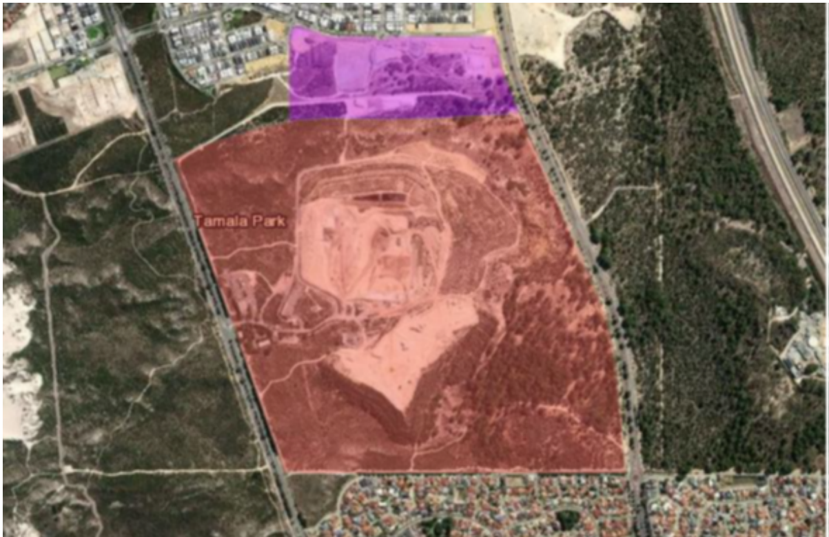
Plate 5: Current CS Act classified areas as shown in the Contaminated Sites Database DWER (2023), with red area classified as 'Contaminated – Remediation Required' and the pink area classified as 'Contaminated – restricted Use'.
